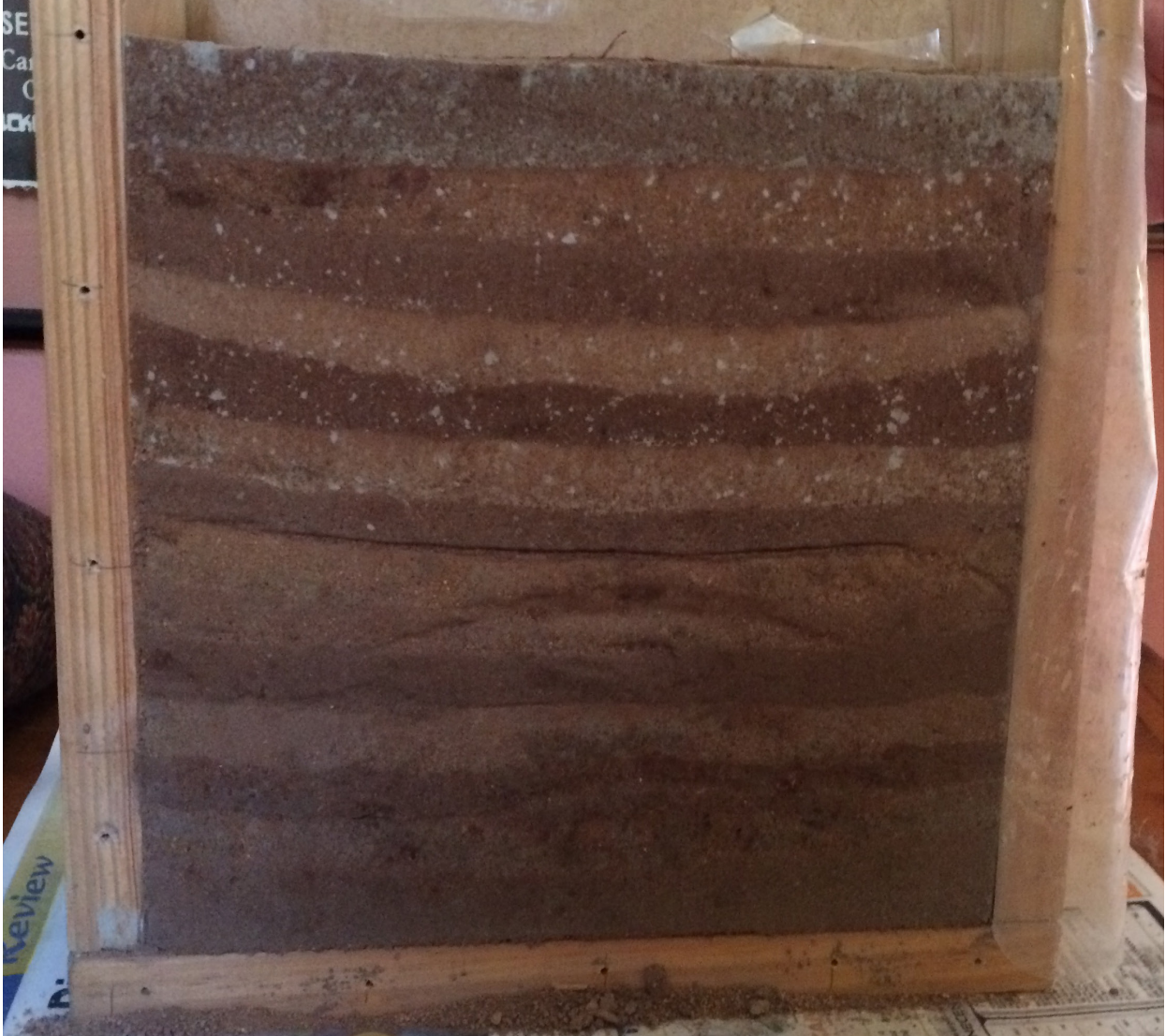
Experimenting with different grades of rammed earth with different mixtures of clay cement and sand.
