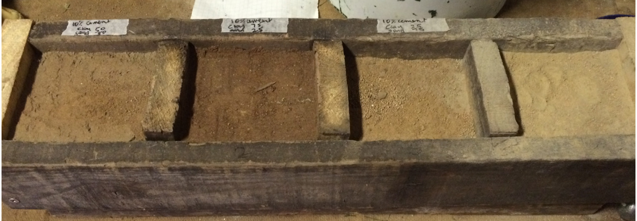
Experimenting with different grades of rammed earth with different mixtures of clay cement and sand.
