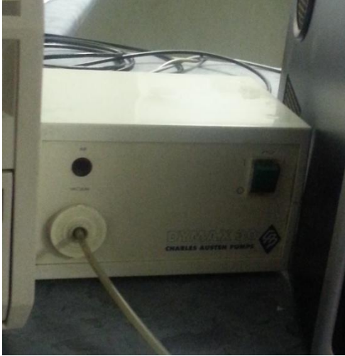
Fig 6: Vacuum pump CBCT
