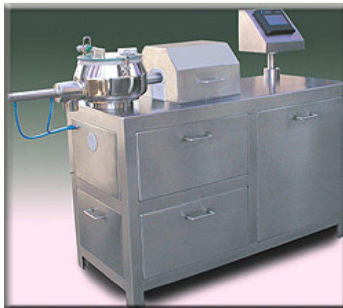
Figure 3.1: Saral Rapid Mixer and wet granulator R&D model
