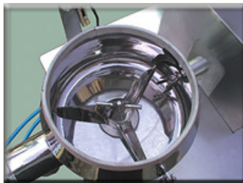
Figure 3.2: Mixer blades of Saral Rapid Mixer and wet granulator R&D model
