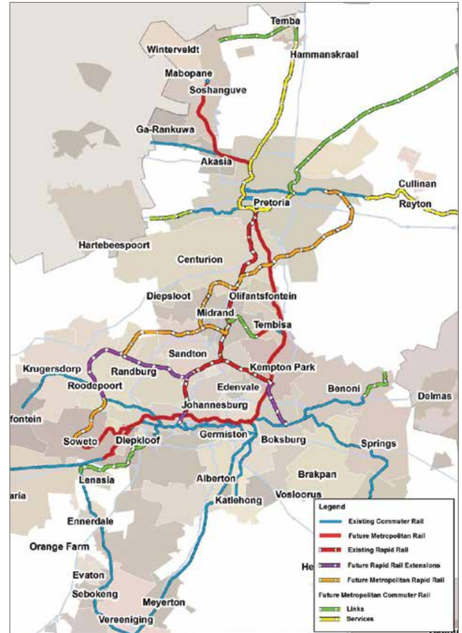
Figure 1.2: ITMP25 proposed railway network (Source: GDRT, 2013a, p.42)
