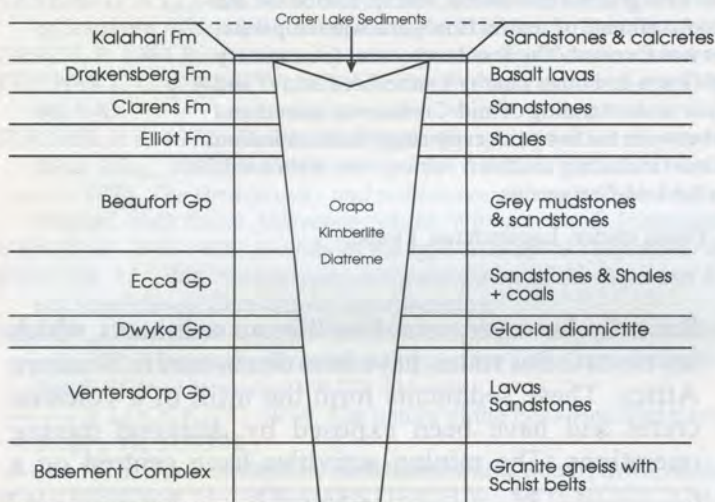
Figure 2. Generalised geological section of Orapa diamond mine.
