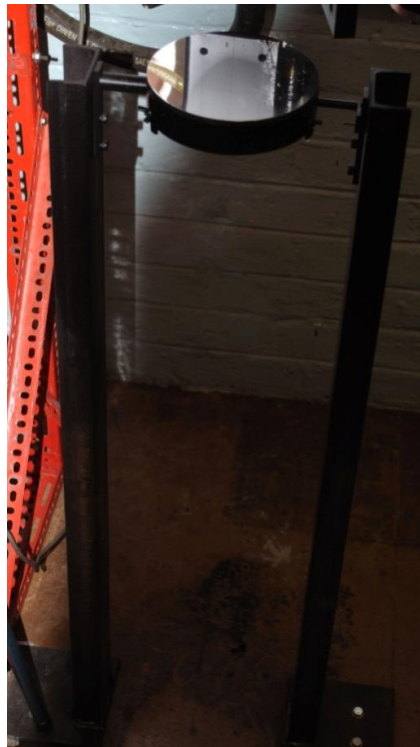
Figure 4-3: Photograph of the impingement plate mount with aluminium impingement plate
