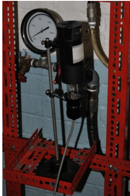
Figure 4-4: Photograph of sodium lamp with shroud
