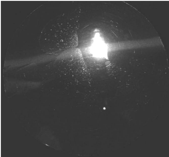
Figure 6-4: Oil Film Coating After Impingement
