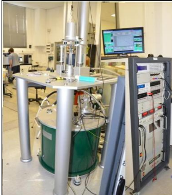
Figure 4.6: Cryogenic measurement system for low temperature electronic transport characterization of SWNT mats from 2 – 300 K in the presence of a magnetic field 0– 12 T
