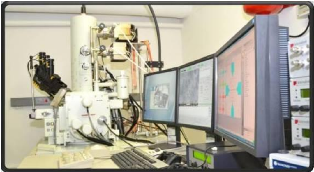
Figure 4.1: JEOL 7001F SEM facility used structural characterization of the synthesis. It is coupled to a gas injection system and nano-manipulators operated with at acceleration voltage up to 15 kV.
