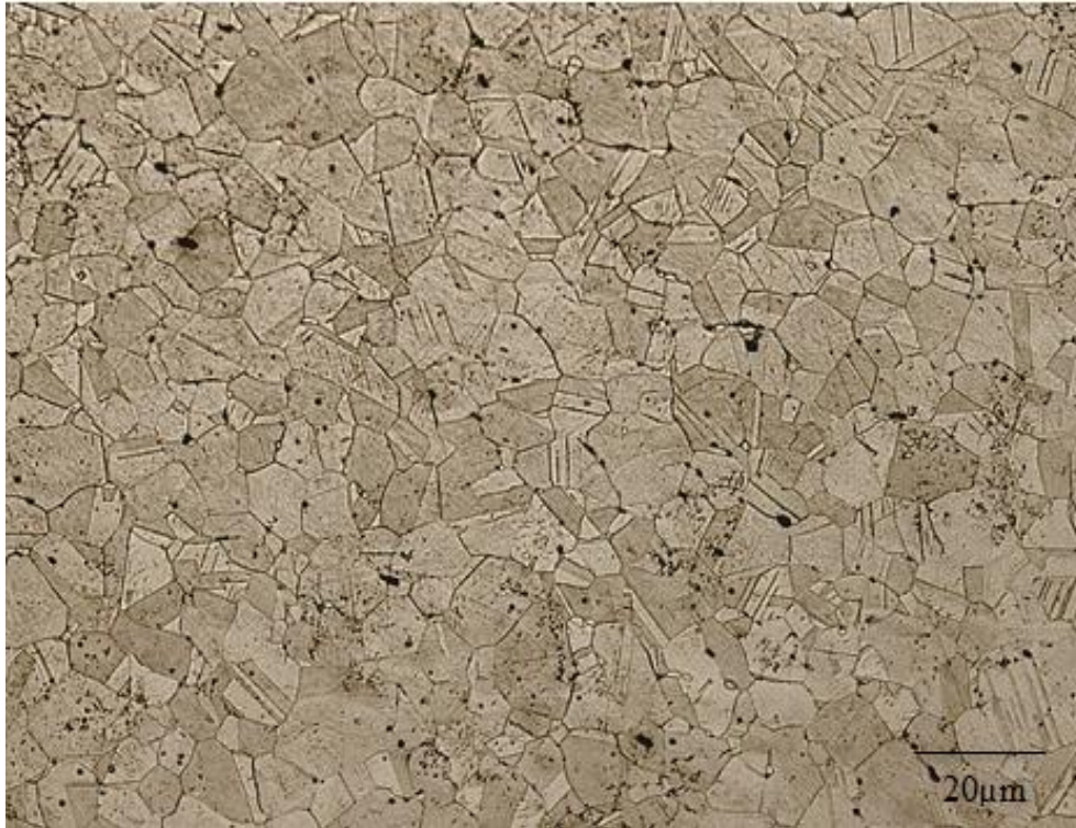
Figure 4.7. Micrograph of the core of as-received rolled AISI 316L steel.
