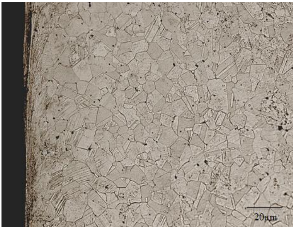
Figure 4.8. Micrograph showing the surface of as-received rolled AISI 316L steel.
