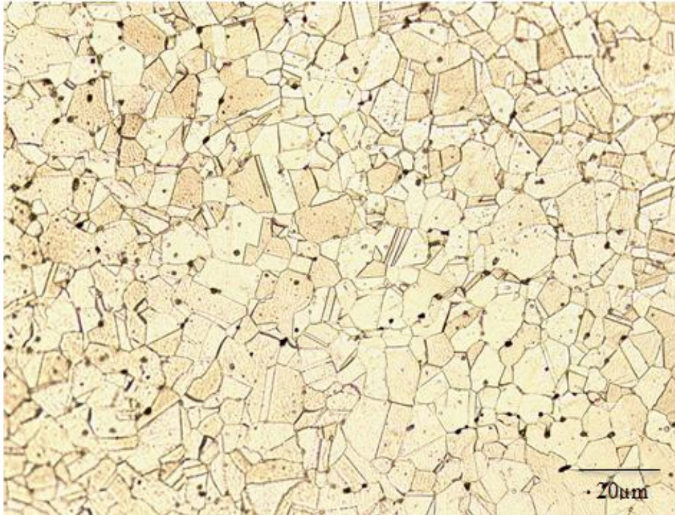
Figure 4.13. Micrograph of the core of AISI 316L steel carburised at 650°C.
