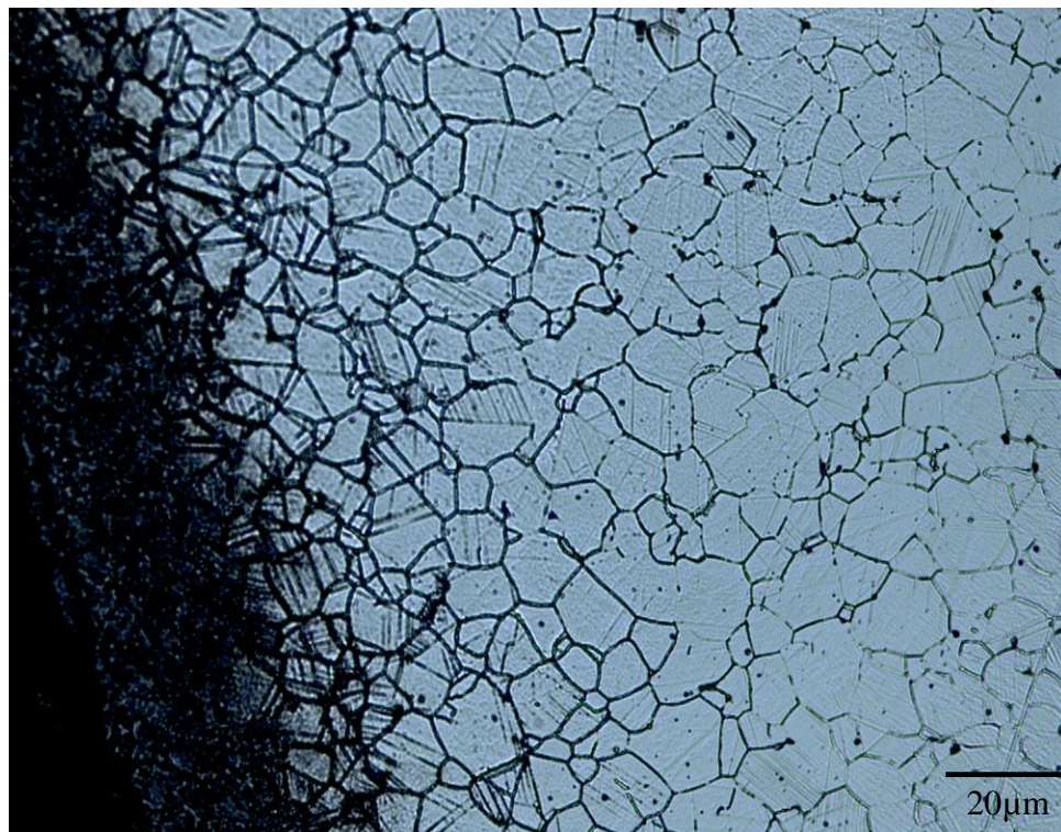
Figure 4.16. Micrograph showing the surface of AISI 316L steel carburised at 700°C.
