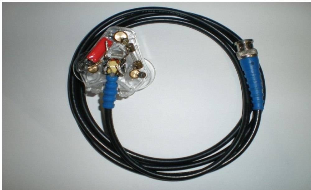
Figure 3.5: Coupling Circuit Showing the Final Termination with a BNC Connector.
