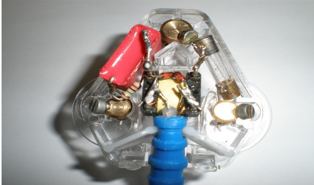
Figure 3.4: Coupling Circuit Neatly Packed In a Three-Pin Plug.
