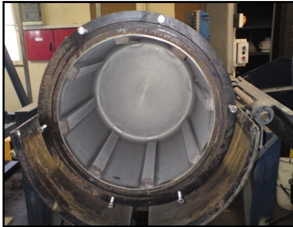
Figure 3.8 Photograph of the laboratory mill showing the lifters
