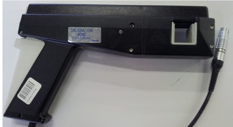
Figure C.1: Current probe used to measure three-phase rectifier output to field windings on rotor
