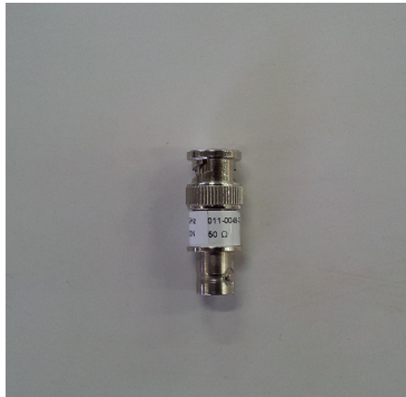
Figure C.3: BNC termination (feedthrough) used to connect amplifier to DSpace controller panel
