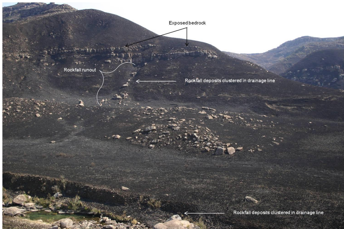
Figure 7.64 Rockfall deposits in the GCSF. Rock movement types include toppling and falling.
