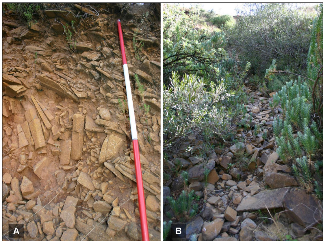
Figure 6.15 (A) Profile of the main scarp. (B) Angular material that is being transported in the flow channel.
