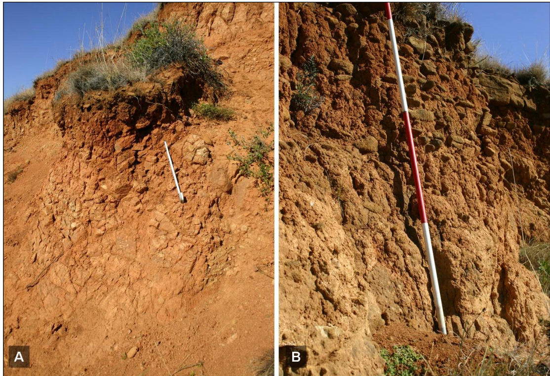
Figure 6.29 (A) Vegetated 'islands' on the shear surface and (B) the gradual transition of the contact between the mobile soil and weathered saprolite.
