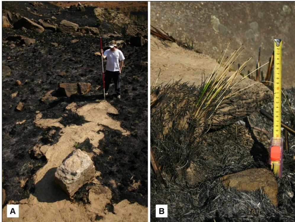
Figure 6.22 The flow deposit at site G indicating (A), how the flow spread around grass tussocks and (B), how vegetation created a cast that moulded the shape of the deposit.
