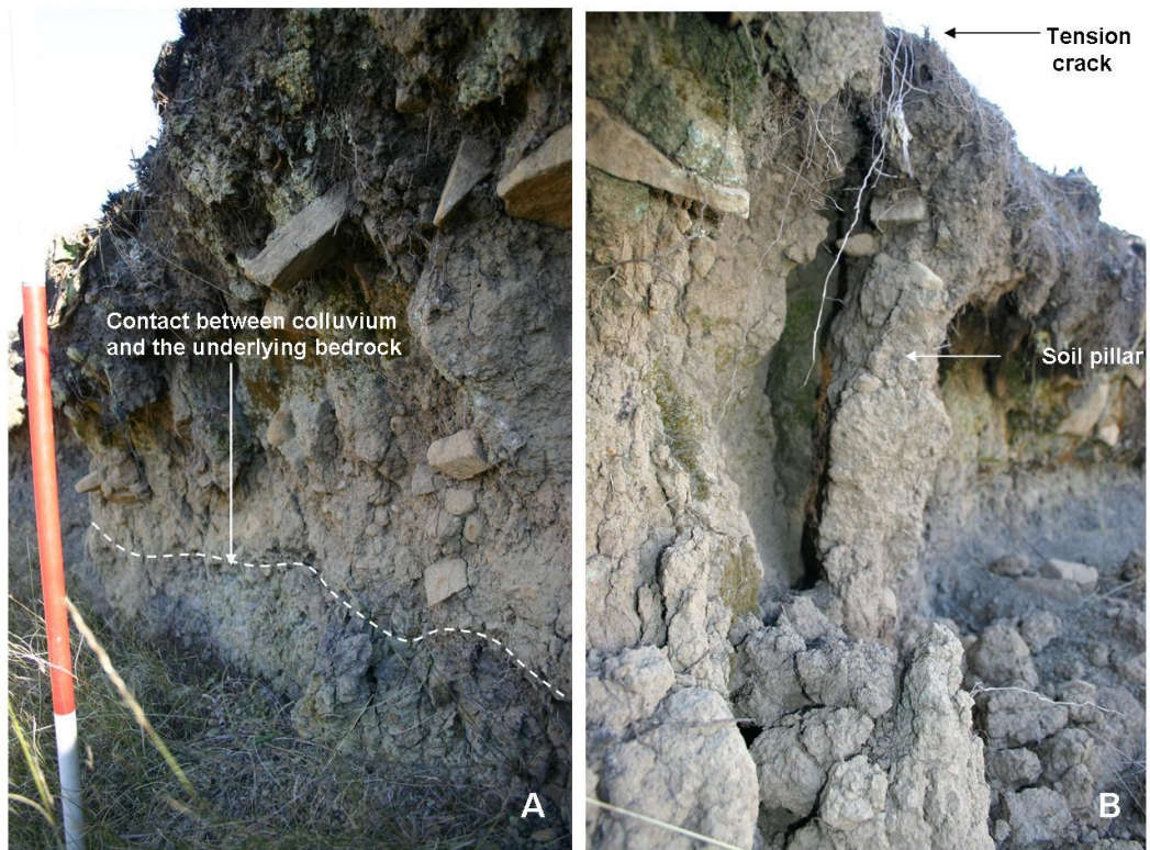
Figure 6.4 (A) The contact between the colluvium and mudstone and (B) a tension crack at the crown of the slide scar which has developed into a soil pillar.
