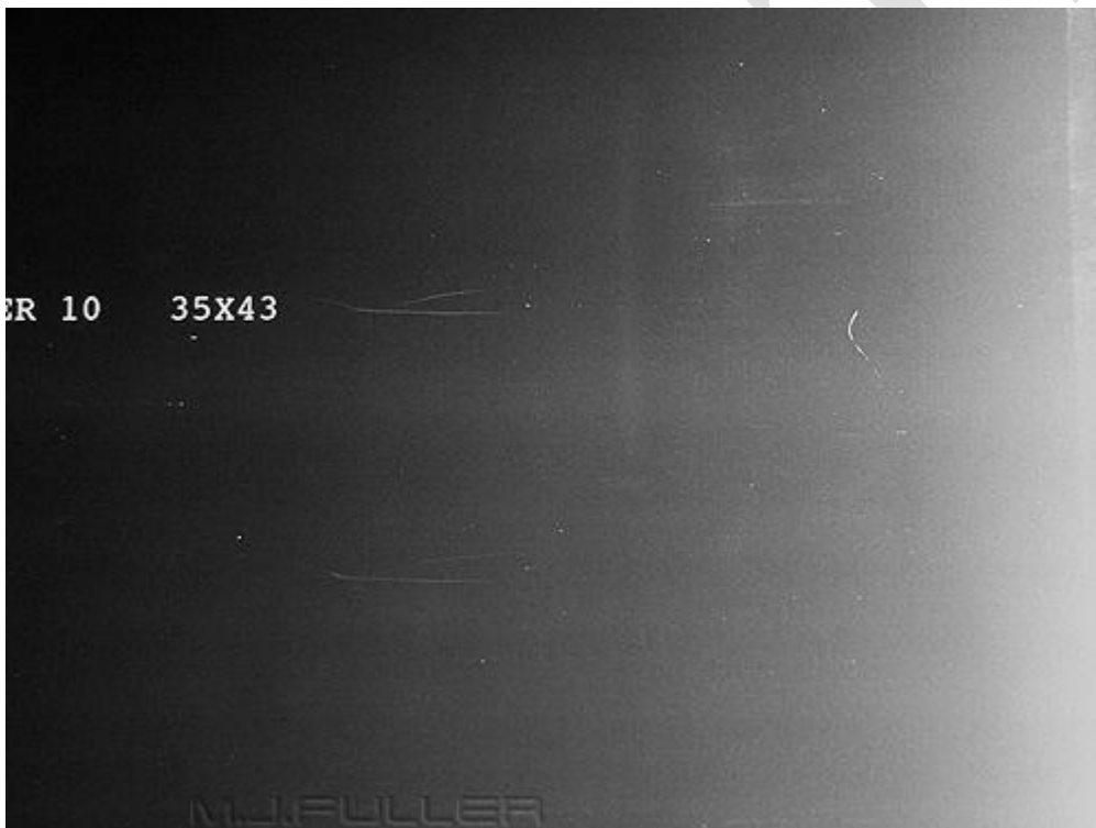
Figure 5.7: A radiograph showing scratch artifacts on a CR image 155 .
