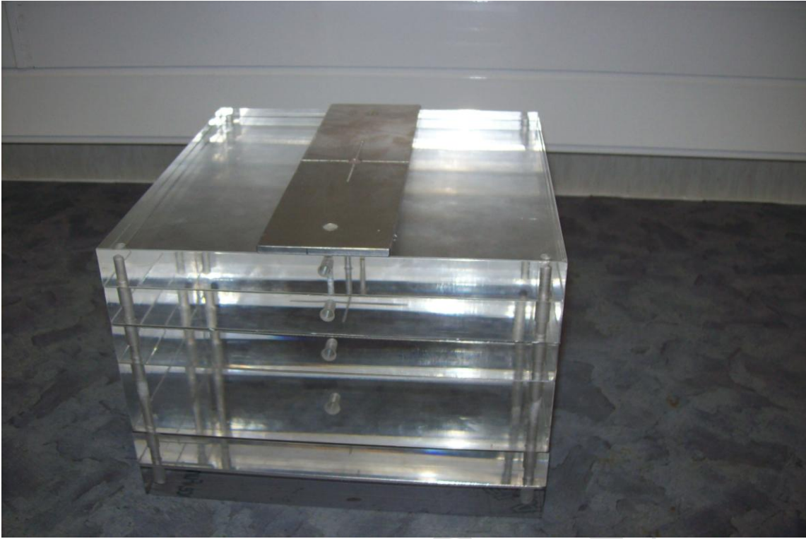
Figure 7.14: A photography of the fabricated ANSI abdomen phantom.
