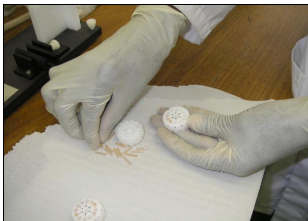
Figure 4.1: Loading cartridges into cartridge holder. Prepared cartridges were stored at 10°C until time of biolistic inoculation.
