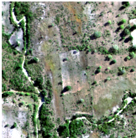
Figure 3.14.: A subset from the CAO scene over the Bushbuckridge area showing trees, grass and water. The RGB image is used in this illustration, with red approximated by band 35, green approximated by band 16, and blue approximated by band 10.
