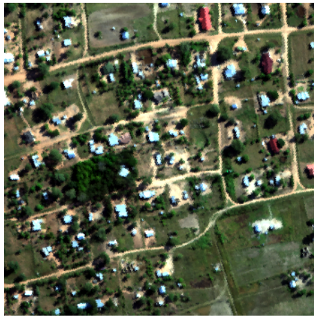
Figure 3.13.: A subset from the CAO scene over the Bushbuckridge area showing houses, roads and fields. The RGB image is used for this illustration, with red approximated by band 35, green approximated by band 16, and blue approximated by band 10.
