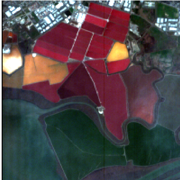
Figure 3.8.: A subset of the 2011 Hyperion scene over Moffet Field, California, USA. The RGB image has been used in this illustration, with red approximated by band 26, green approximated by band 9, and blue approximated by band 3.
