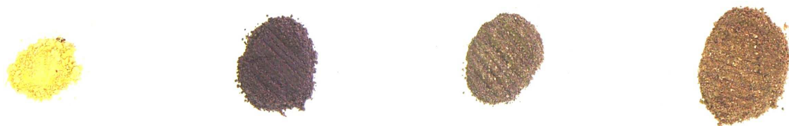
Figure 4.4: Unheated sample (left), 200°C, 300°C and finally 400°C (far right) The samples shown are 5% Au-1% Pt on silica. In all cases the different colours can be attributed to the samples optical absorption in the visible region of the spectrum which is due to the relativistic lowering of the gap between the 5d band and the Fermi level, without this effect the gold nanoparticles would be a white/silver colour and have the same propensity to tarnish and corrode 8 .
