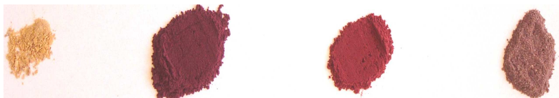
Figure 4.3: Various samples supported on silica prepared and heated under different conditions. Unheated sample (left), 200°C, 300°C and finally 400°C (far right). All samples are 5% Au on silica.
