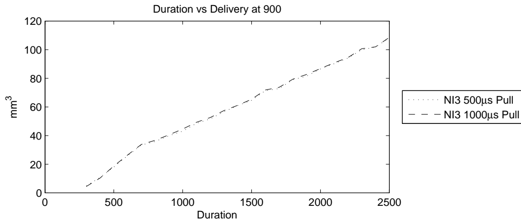
Figure 5.16: Volume of fluid delivered vs injection duration for 500µs and 1000µs Pull Phases, for injector NI3 at 900 bar
