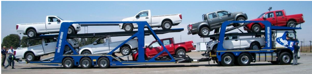
Figure 3.45: A Vehicle Delivery Services Volvo FM400+Maxiporter PBS car-carrier combination (10 m wheelbase trailer)
