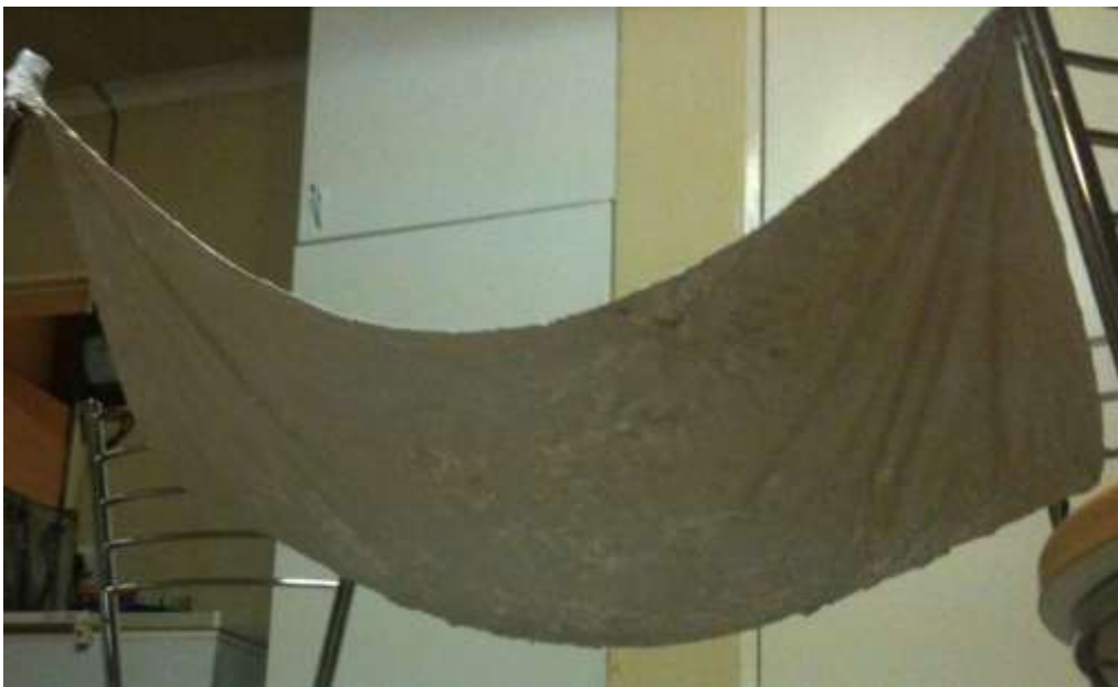
Figure 3: A hanging plaster of Paris mould without wood stiffeners
