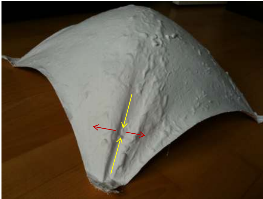
Figure 1: Illustrative display of the internal forces in a free-hanging structure. The yellow arrows indicate tension and the red arrows indicate compression in the structure.
