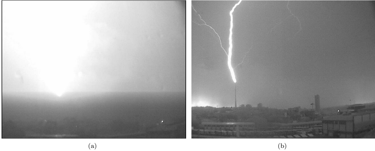
Figure 4: Positive strikes to the tower as recorded by the surveillance (a) 2010-01-07 (b) 2010-04-20.
