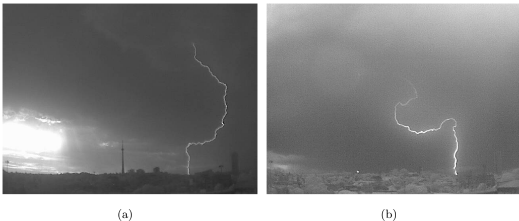
Figure 3.2: Demonstration of downward negative flashes that appear to be intercepted by upward leaders from the ground. This is demonstrated by a sharp change of direction in the channel path.
