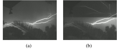
Fig. 3: Consecutive images with 10 ms time separation taken of a cloud-to-cloud (CC) lightning strike.
