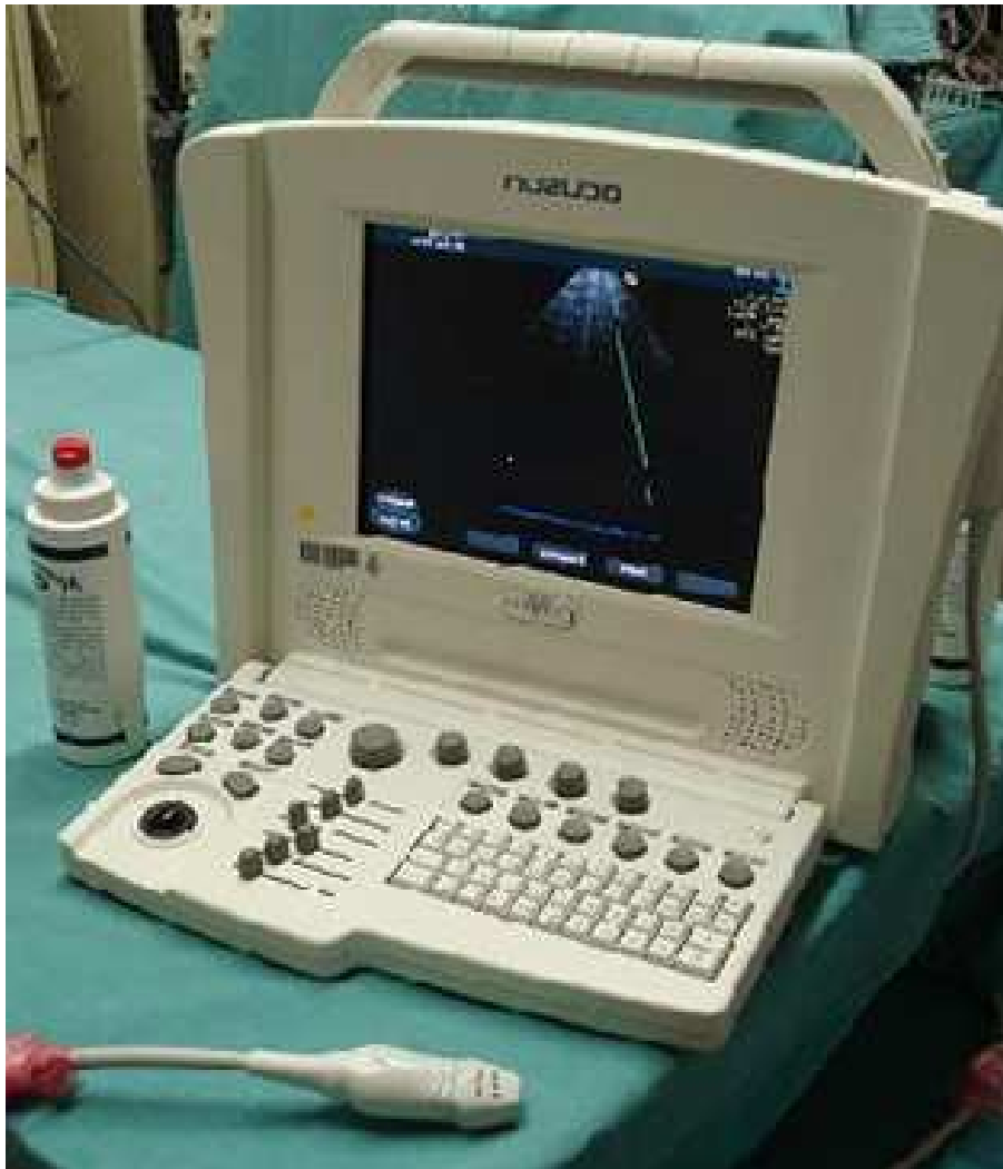
Figure 2.1 ACUSON CYPRESS portable echocardiograph used to obtain in-vivo measures of left ventricular structure and function in anaesthetised rats.
