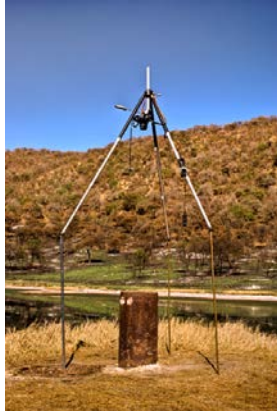
Fig. 40 Camera on stilts . Photographing down the residual borehole left by T.C. Partridge's drill core
