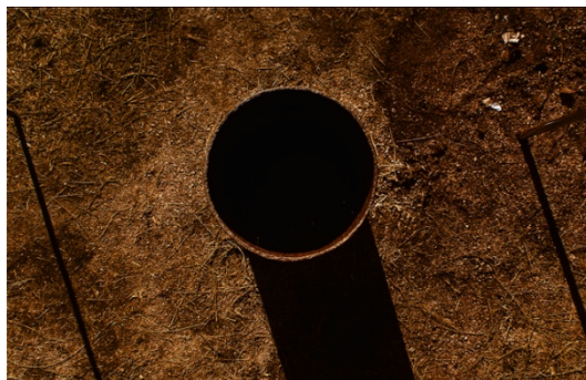
Fig. 41 View through the lens of the camera into the borehole . The surrounding earth is a granite-derived sand
