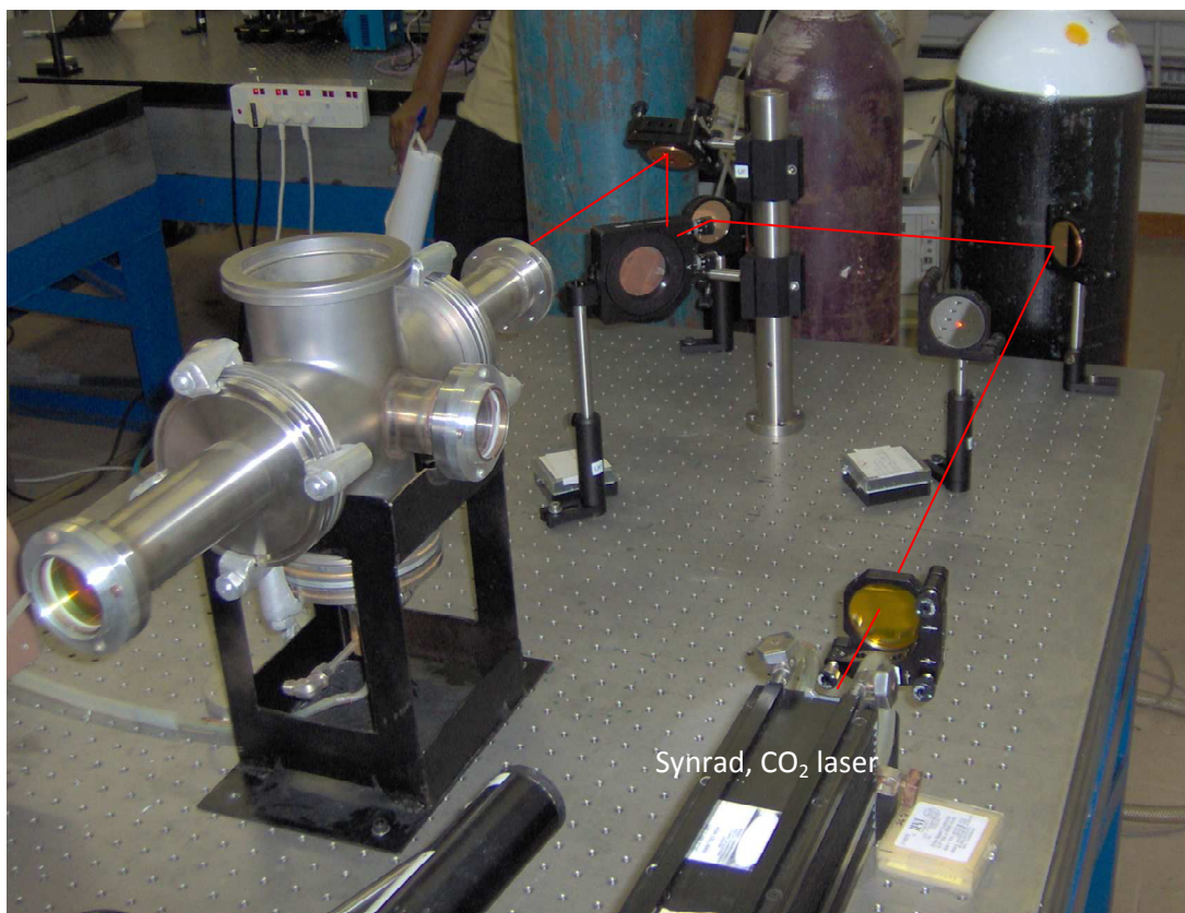
Figure 5.3: Optical layout of the laser pyrolysis experiment showing the delivery of the focused CO 2 laser beam into the reaction chamber.
