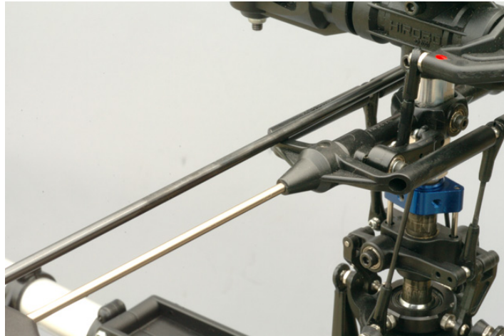
Figure 2.2: Helicopter stabilizer bar
