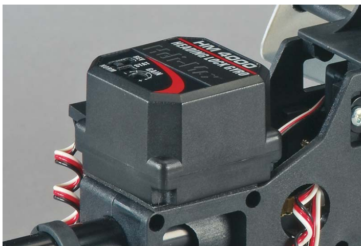
Figure 2.4: Helicopter Yaw Gyro
