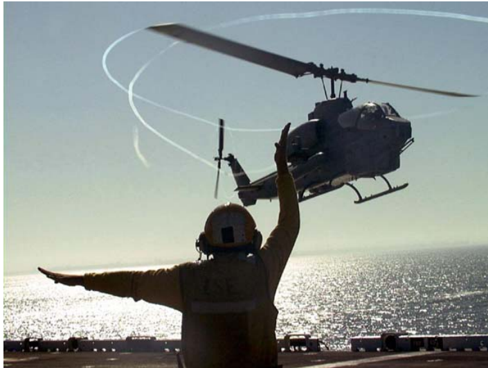
Figure 3.1: Helicopter rotor wake.
