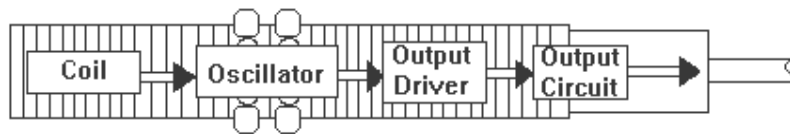
Figure 3.3: The schematic representation of the salient components and operating principle of the inductive proximity sensor.
