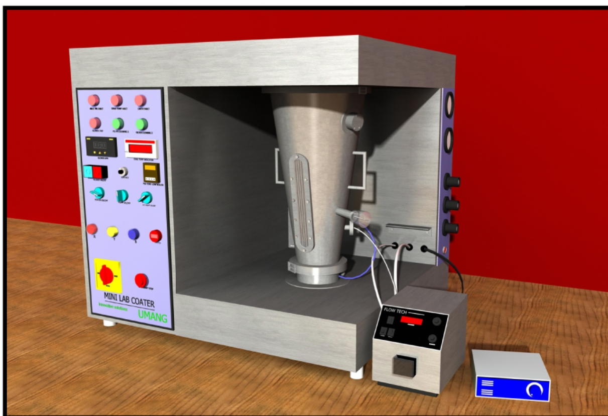
Figure 5.3: Three-dimensional illustration of the fluid bed dryer (FBD) and its components.
