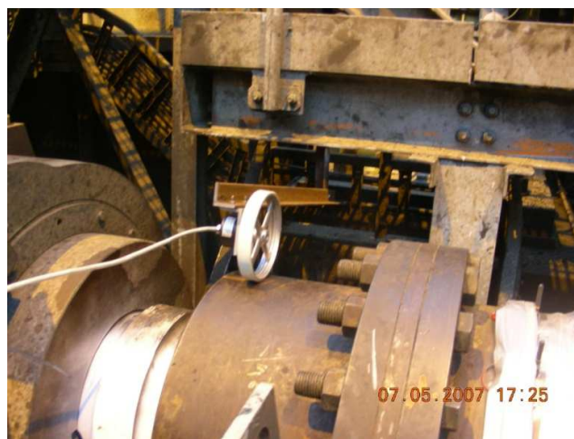
Figure 8 Speed Measurement by means of Tachometer
