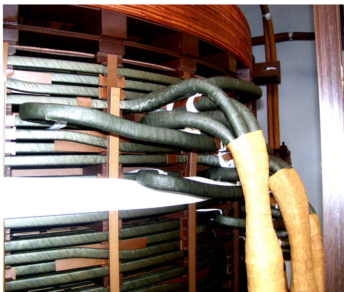
Figure 1 : Transformer solid insulation system in a winding block.
