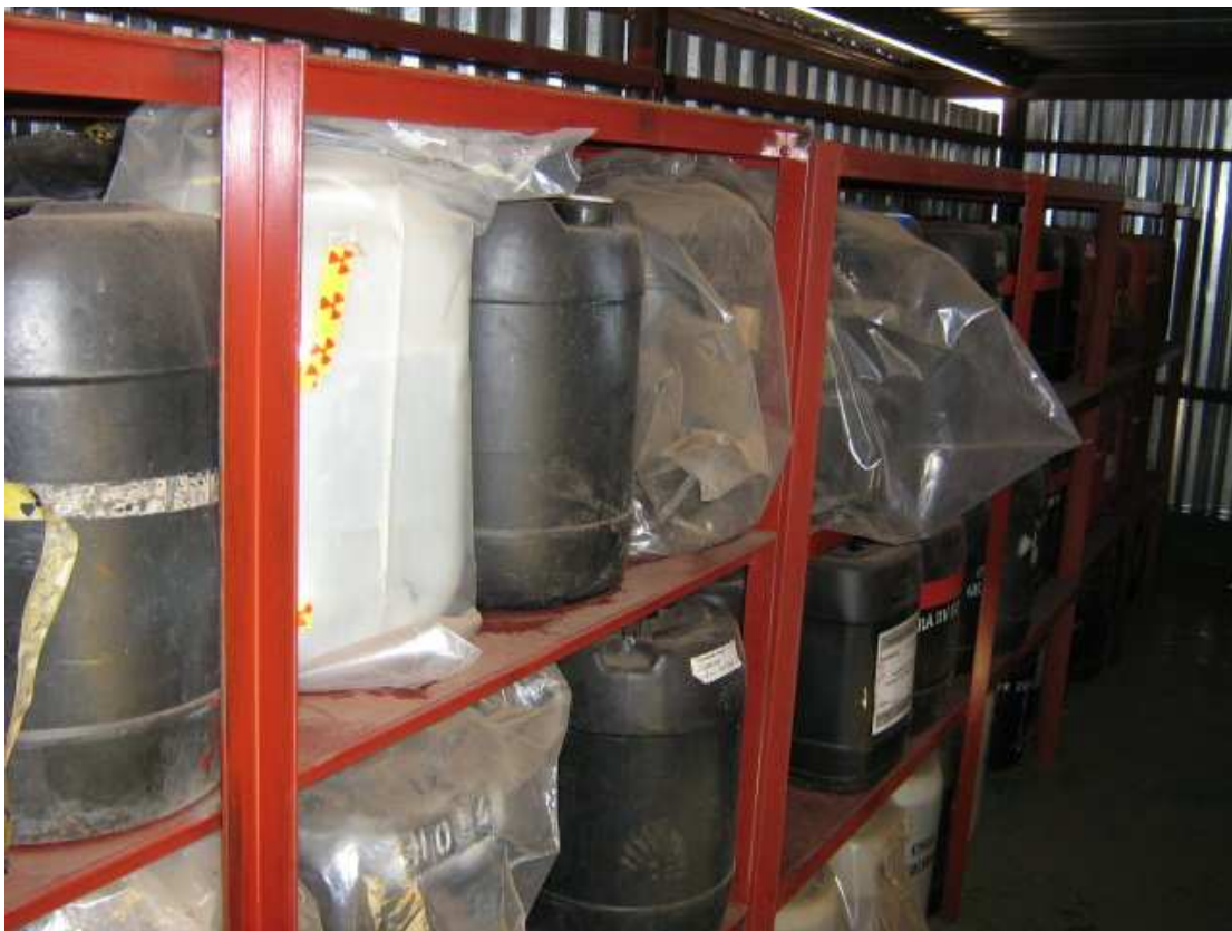
Figure 1.2 Storage of radioactive liquid organic waste in high density polyethylene containers in a secure area with liquid containment facilities
