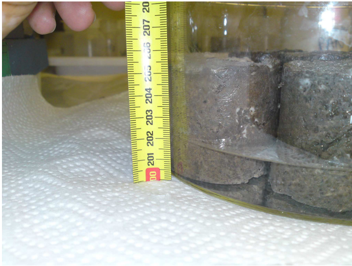
Figure 3.9 Sorptivity measurements with bottom side and top sides of samples not coated with vacuum grease
