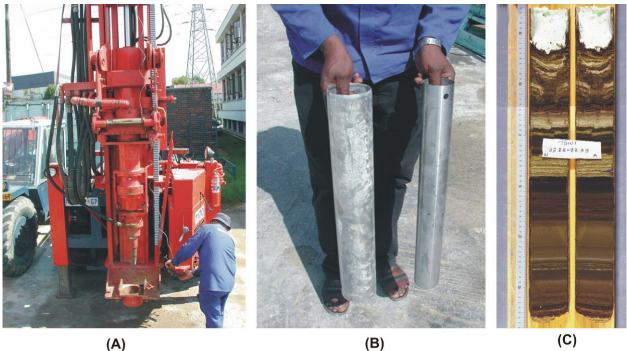
Fig.7. A: Soiltech driller, B: Shelby tube drilling and C: TSW-1 core sediments (Kristen, 2009)
