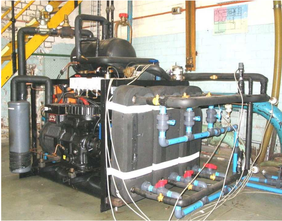
Figure 3.6: The experimental equipment of the refrigerant evaporator tests
