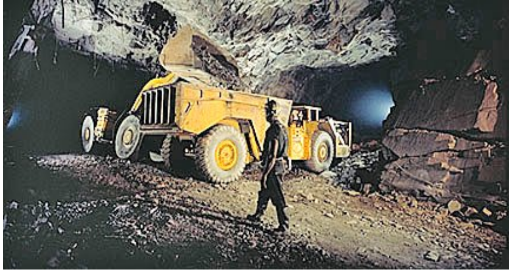
Figure 4.3 A Scoop loading into a dump truck underground
