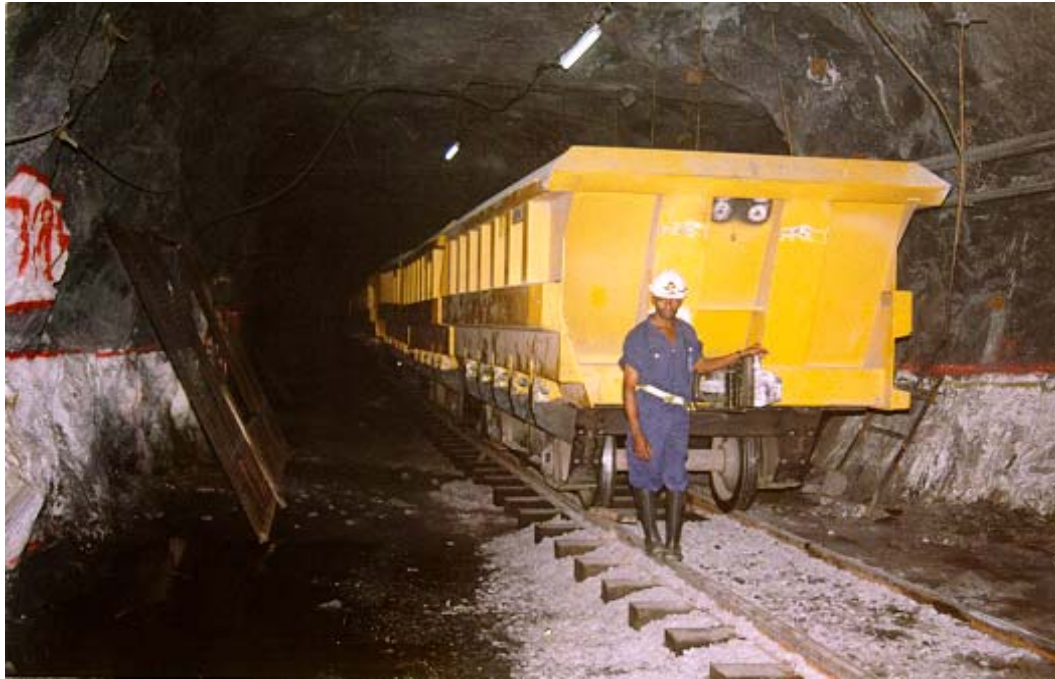
Figure 4.4 20-tonne bottom dump loco truck on 41 Level
