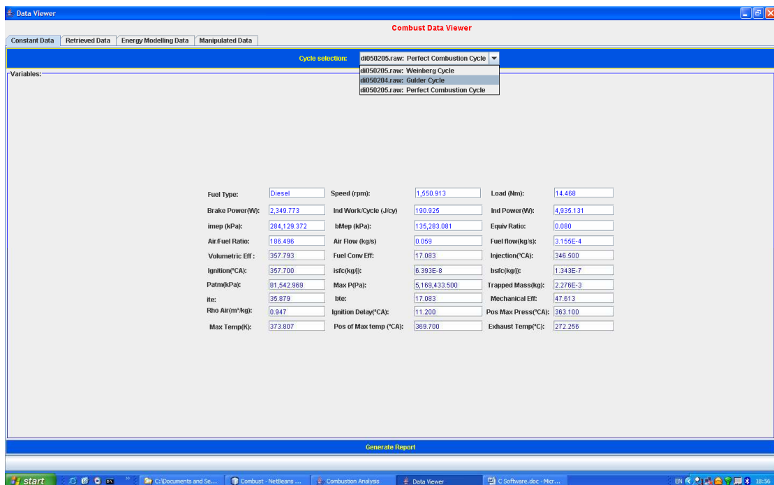
Figure C13: The Data Viewer GUI illustrating the Constant Data Tab and Drop down Engine Test Selection box
