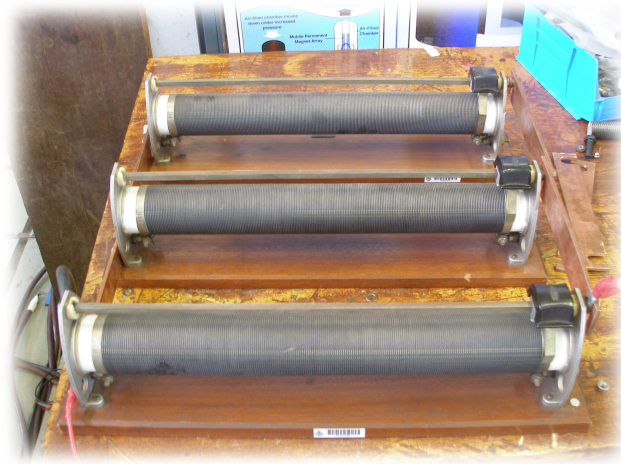
Figure 5.9: The rheostat arrangement was used to produce full-load current densities of 5\text{A}/\text{mm}^2 in each of the stators from a single DC generator supply.
