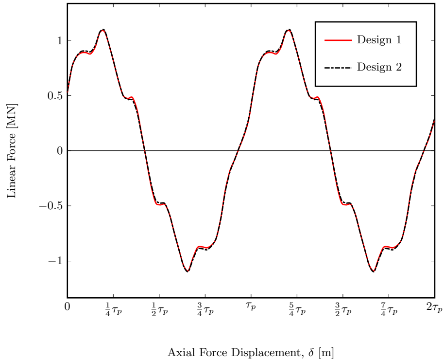
Figure 5.5: Full-scale Designs' Force Distributions (Plot Peaks of 1.089 MN and 1.090 MN respectively).
