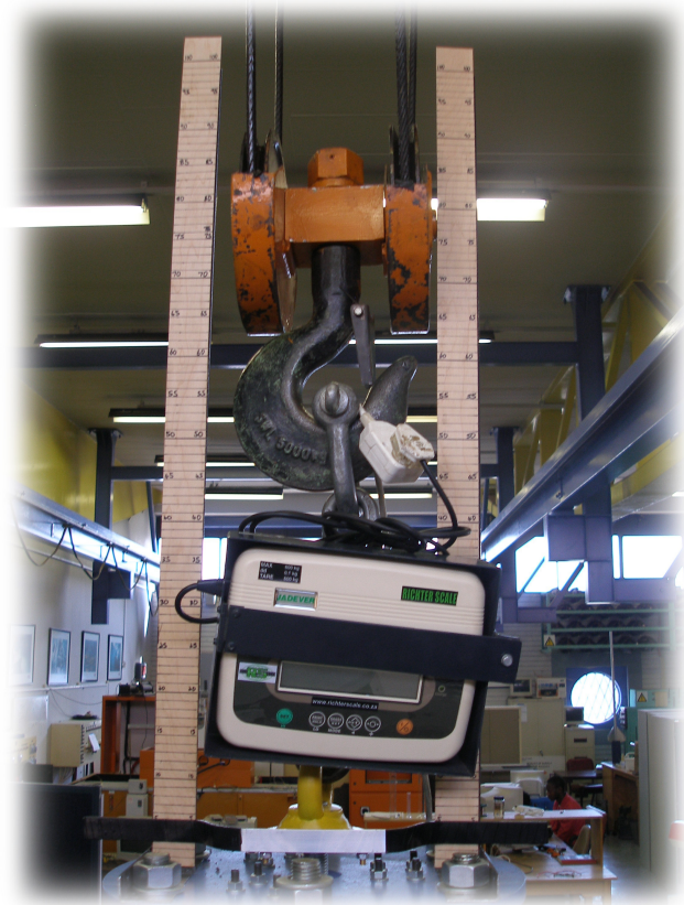
Figure 5.10: Static Force Testing Apparatus. The load-cell based scale measured the force exerted on the translator by the stator field, which opposed the upward force that the crane exerted on the translator.
