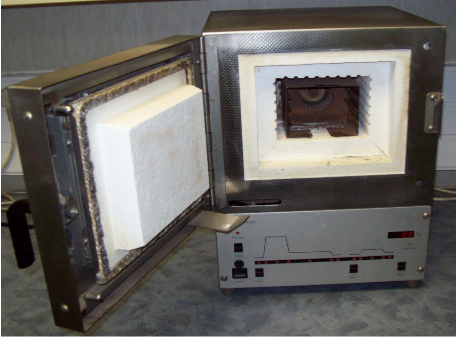
Figure 5: The Oven used to anneal the TLDs
