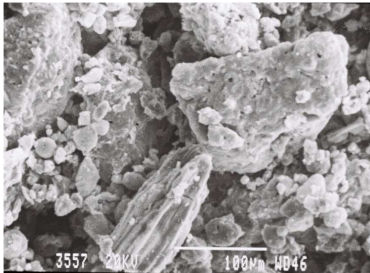
Fig. C.14 Morphologies of char particles at 1400 °C (20% sawdust)
