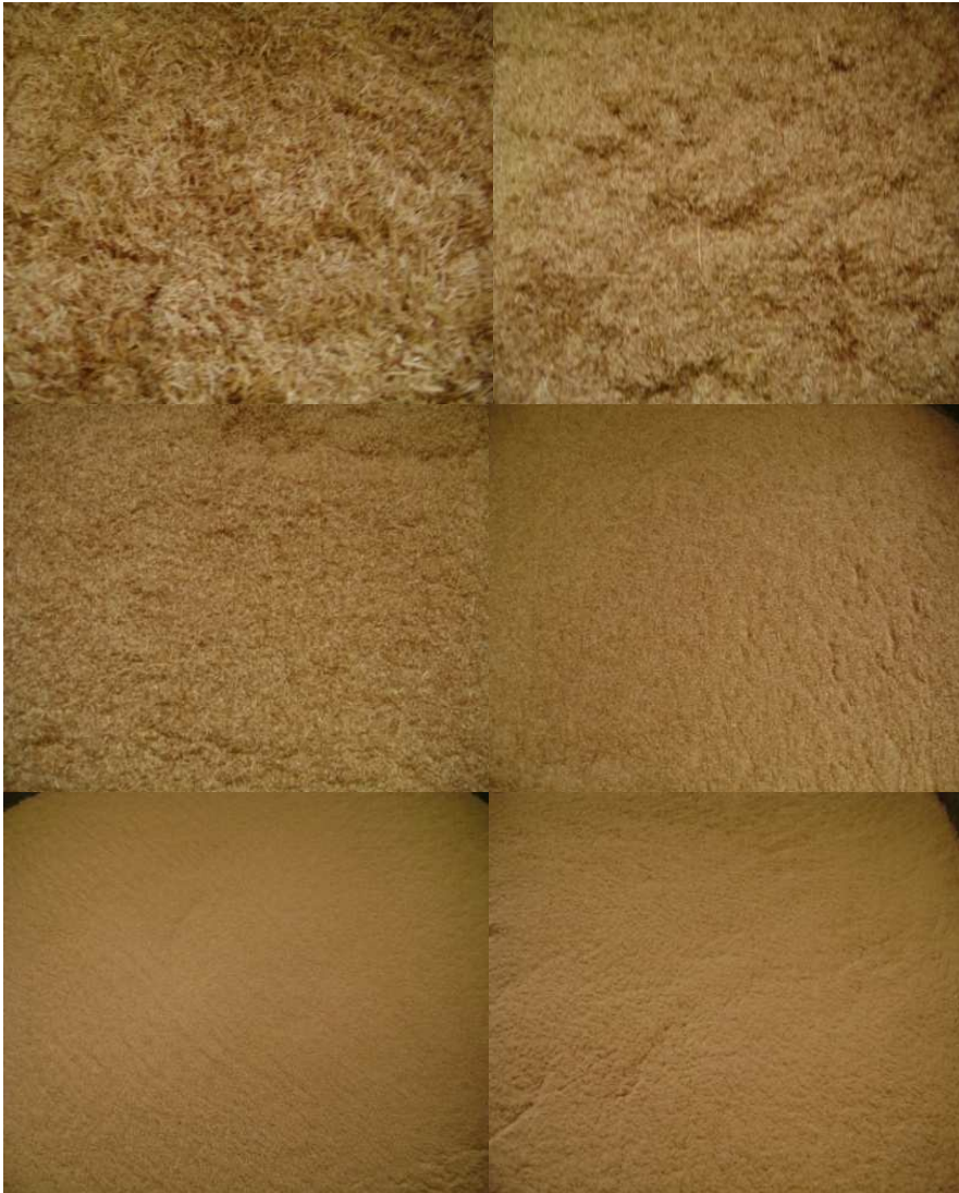
Fig. 3. 8 Sawdust fractionated into size grades respectively 3 – 1 mm, 1 – 0.5 mm, 500 – 212 \mu\text{m} , 212 – 106 \mu\text{m} , 106 – 75 \mu\text{m} , and – 75 \mu\text{m} from top to right.
