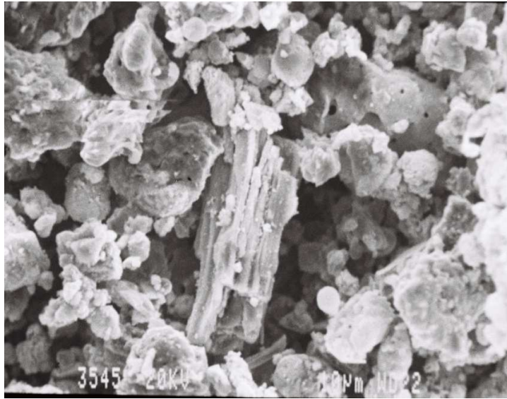
Fig. C.13 Morphologies of char particles at 1400 °C (15% sawdust)
