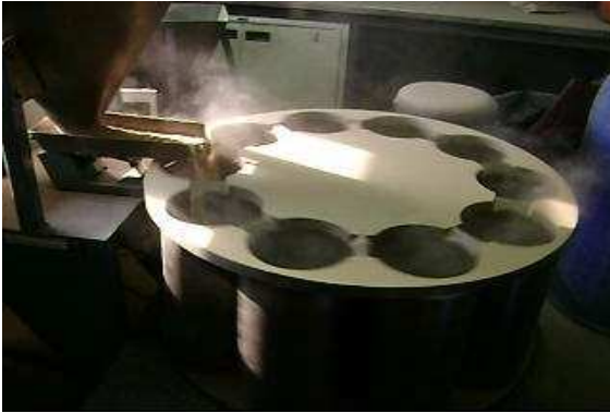
Fig. 3. 9 The splitter used to mix or subdivide samples
