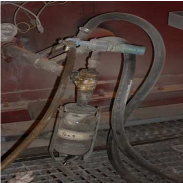
Fig. 3. 6 Back end of the Suction pyrometer inserted at port 9 of the PSCTF
