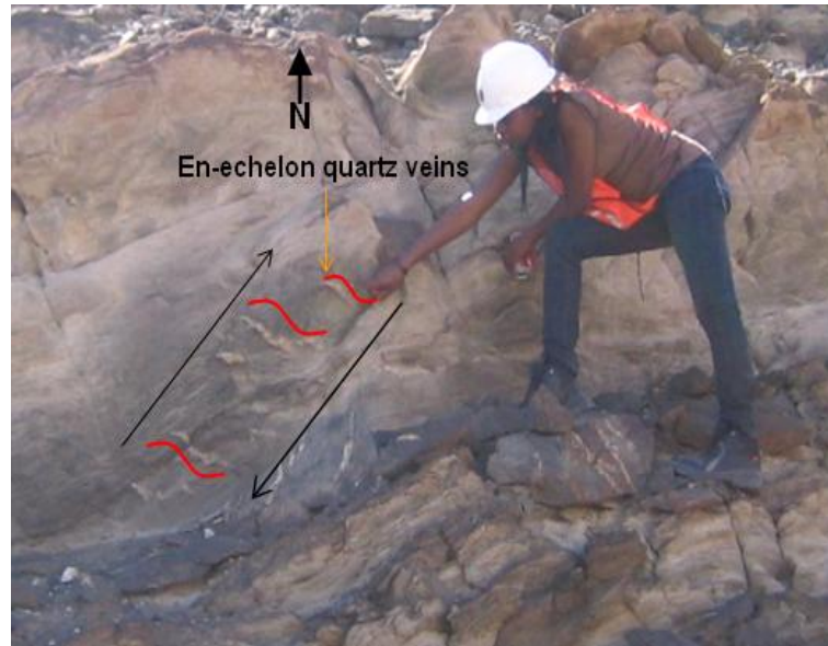
Figure 4.7: En-echelon quartz veins within banded gneiss, indicating a dextral sense of movement.
