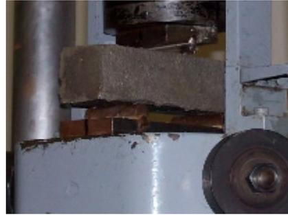
Loaded sample during flexural strength test
