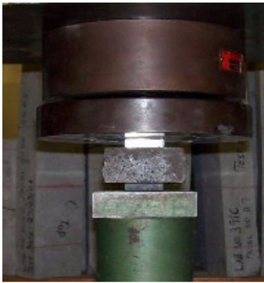
Loaded sample during mortar compressive strength test
