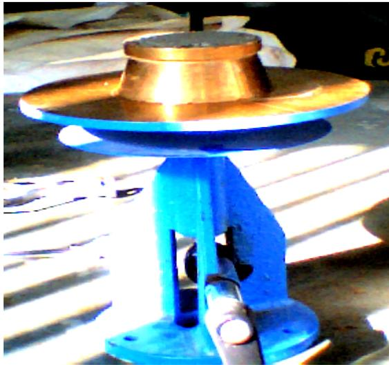
**Figure 3.1: Flow table and sample during testing.**
