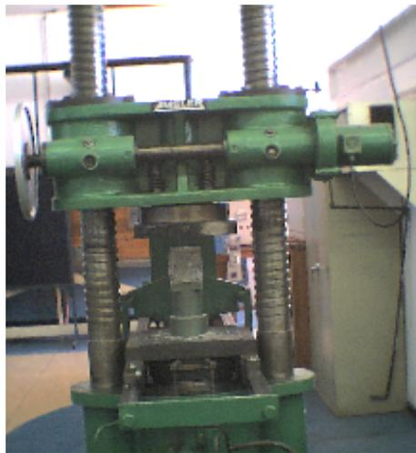
Amsler compressive strength testing machine
