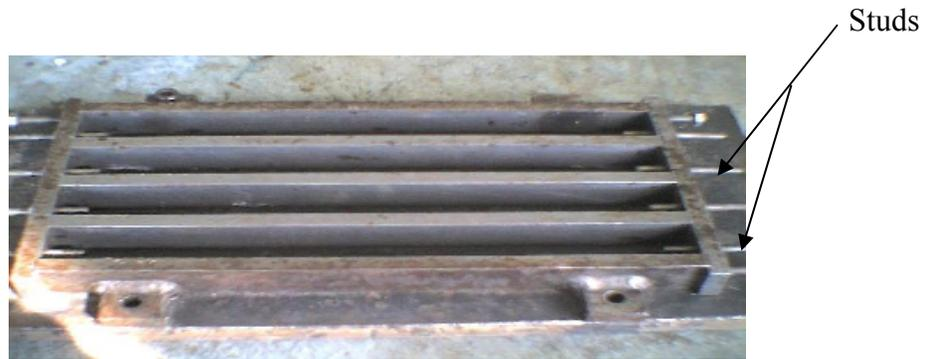
**Figure 3.5: 25 x 25 x 280 mm prism mould with attached studs.**
