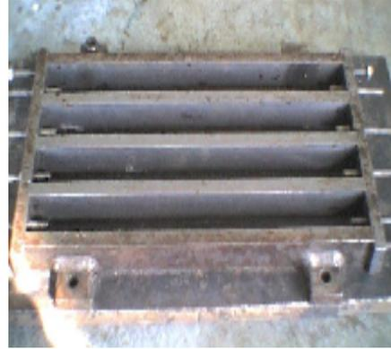
25 x 25 x 280 mm prism mould
