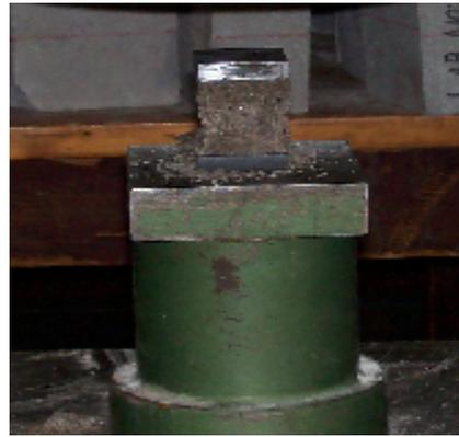
Failed sample after compressive strength test
