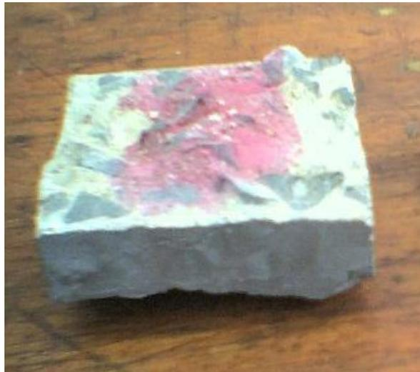
**Figure 3.10: Partly carbonated sample**
