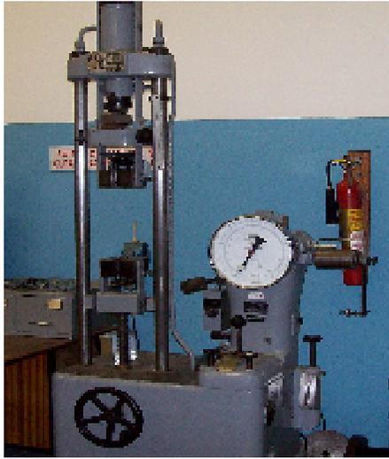
Tensile strength testing machine
