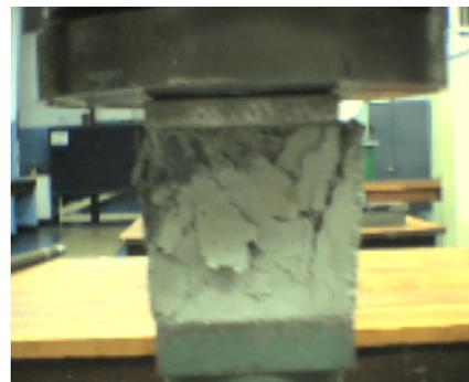
Failed sample after compressive strength test
