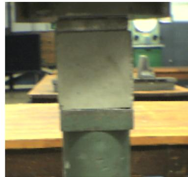
Loaded sample during concrete compressive strength test
