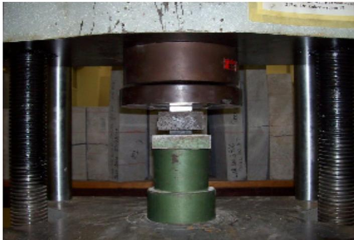
**Figure 3.3: Placement of sample in compression testing machine**
