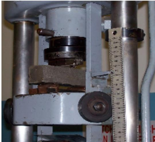
**Figure 3.2: Placement of sample in flexural testing machine**
