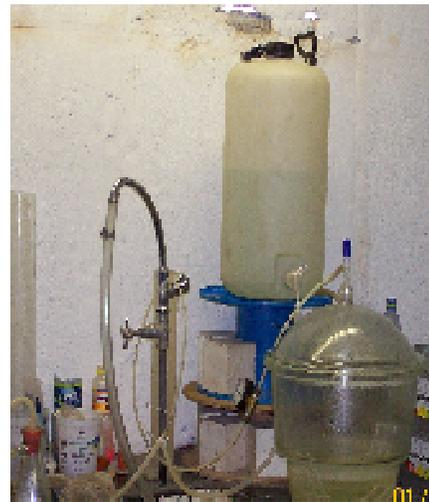
Sorptivity test set up
