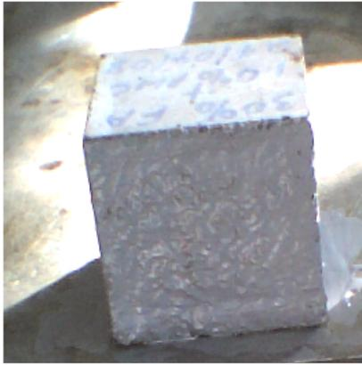
Sample covered with epoxy before carbonation test
