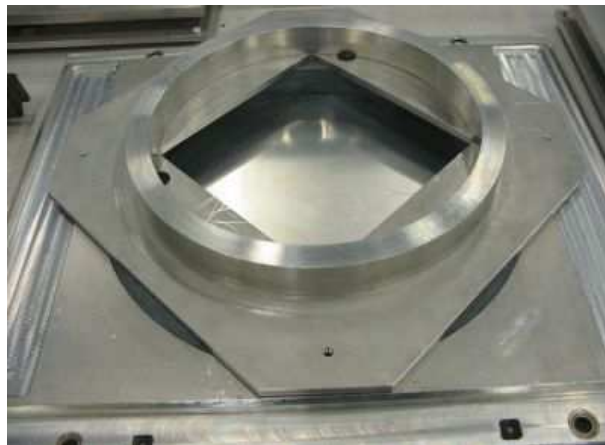
Figure D.3: Plate constructed to match the circular bearing
