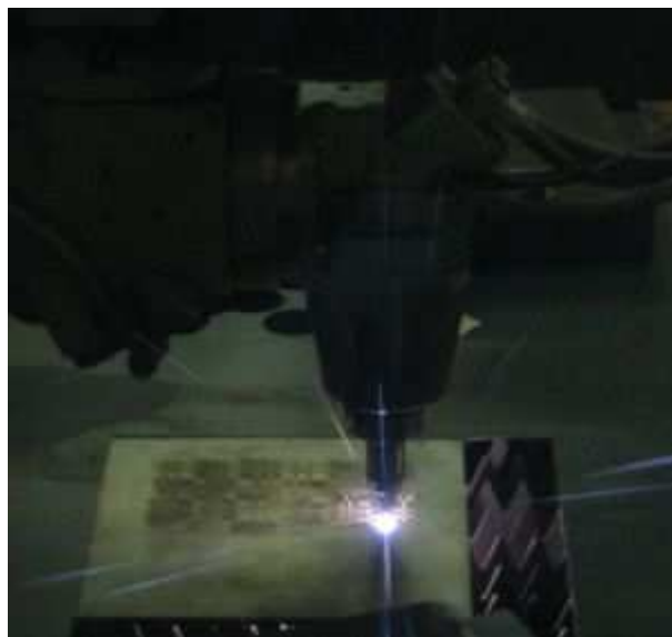
Figure D.10: Laser drilling of a 1 mm tungsten sheet
