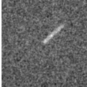
Figure 6.16: Acquired syringe source, highly transparent aperture, 285 counts
