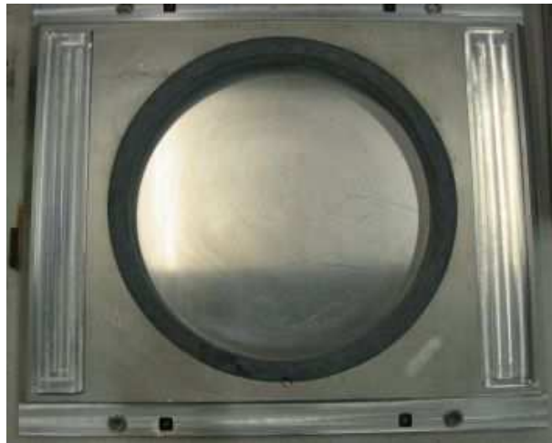
Figure D.2: Circular bearing in the base of the coded aperture frame
