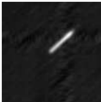
Figure 6.15: Acquired syringe source, opaque aperture, 3270 counts
