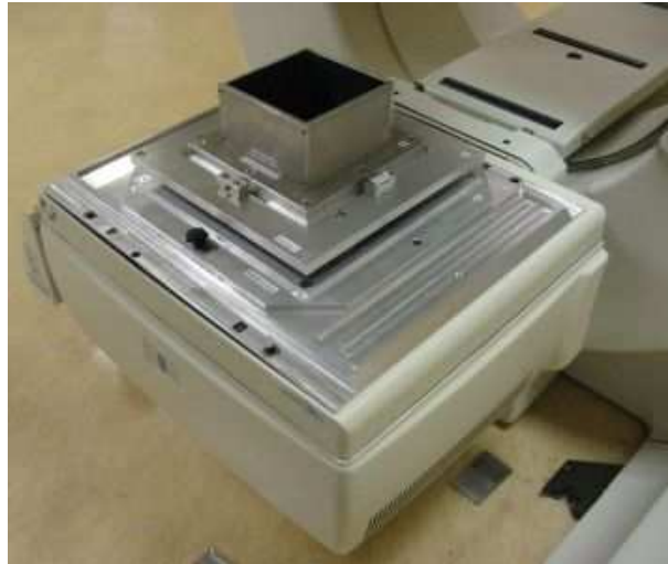
Figure 6.3: Gamma camera frame mounted on the Philips Axis
