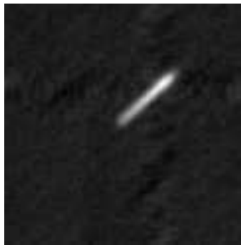
Figure 6.14: Acquired syringe source, opaque aperture, 286 counts
