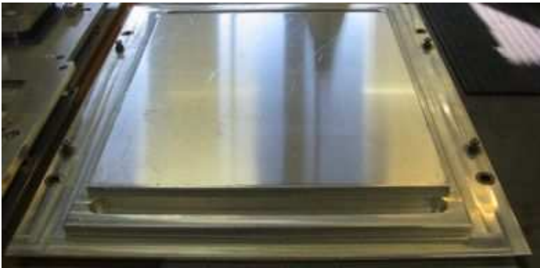
Figure D.1: Gamma camera side of the coded aperture frame
