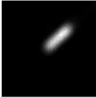
Figure 6.13: Acquired syringe source, LEHR collimator
