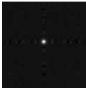
Figure 6.6: Acquired point source, opaque aperture
