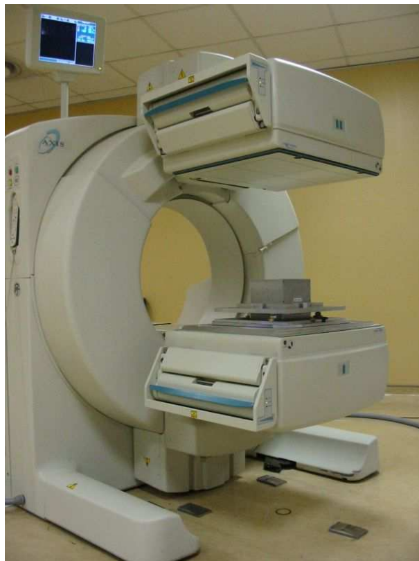
Figure 6.4: Dual gamma camera heads with collimator and coded aperture
