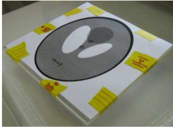
Figure D.11: 2D printed ink and ^{99m}\text{Tc} Shepp-Logan phantom
