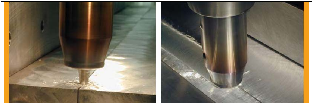
Figure 2.4: Welding tool plunge (left) and transverse (right).
