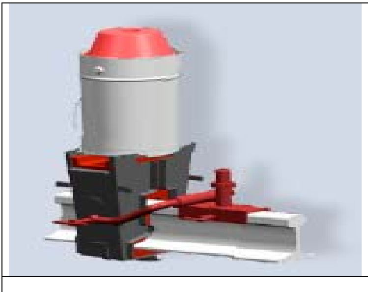
Figure 0.2M: Example of exothermic welding applied on rail
