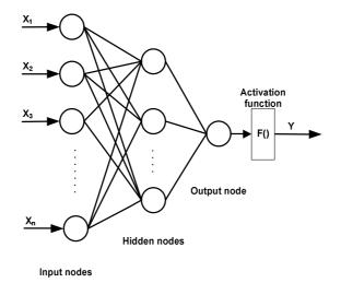
Figure 2.1: The MLP structure showing the inputs, the layers and the activation function [43].
