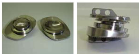
Kineflex metal-on-metal: mechanism, (b) assembled
