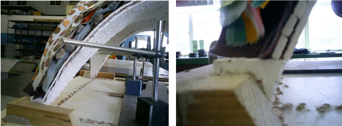
Fig 6-23: Buckling of catenary groin vault
