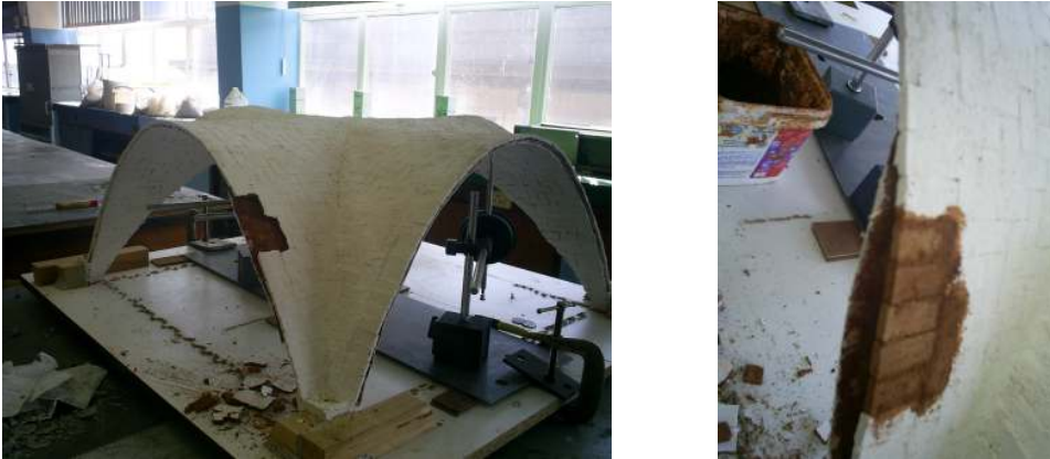
Fig 6-24: Damage and repair to edge of vault
