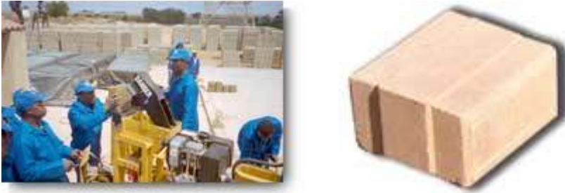
Fig 6-1: Hydraform diesel block press and standard profiled block ( www.hydraform.com : accessed May 2007)
