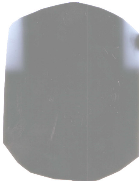
Figure A.2 Shows an exposed film (using a 7 cm x 7 cm field size) at 6 MV for the four field box technique, showing the box shape. Film was cut and positioned in figure 4.10.
