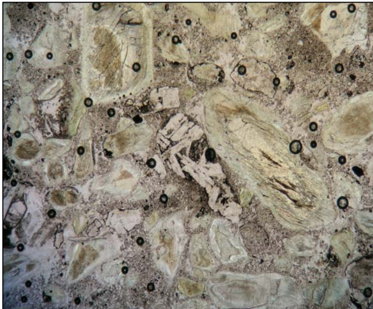
Plate 8: Sample EGG 764, obtained from a depth of 143m in hole PLT008, illustrating the higher levels of alteration compared to a more typical south lobe kimberlite, e.g. Plate 4. Note the serpentinised greenish olivines, and the feldspar-bearing basalt fragment in the centre of the view. Field of view is 3mm wide. Image was taken from Hanekom et al. (2006).
