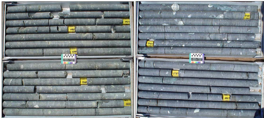
Plate 6: PLT019, ~146.5-159.7m, left, illustrating the texture associated with unit EM/PK(S), showing the small (<1cm) basement fragments. Right – PLT022, ~370-383m, illustrates the appearance of unit M/PK(S). Images from Hanekom and Stiefenhofer (2006).
