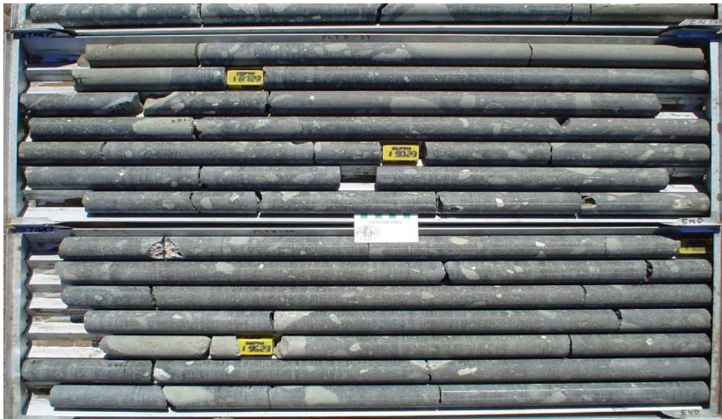
Plate 7: PLT08, ~185-198m, illustrating the texture associated with unit WM/PK(S) in core. Compare this kimberlite with unit M/PK(S), shown in Plate 6. Image from Hanekom and Stiefenhofer (2006).
