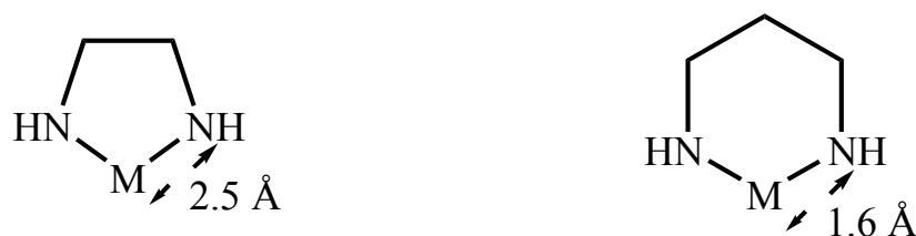
Figure 4.33: The ideal bond lengths for chelate rings with en and tn respectively 15,16
