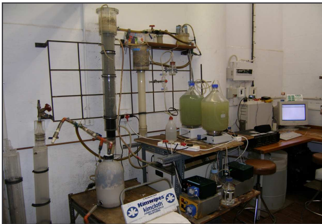
Photograph of the fully automated set up used for biohydrogen production from synthetic wastewater
