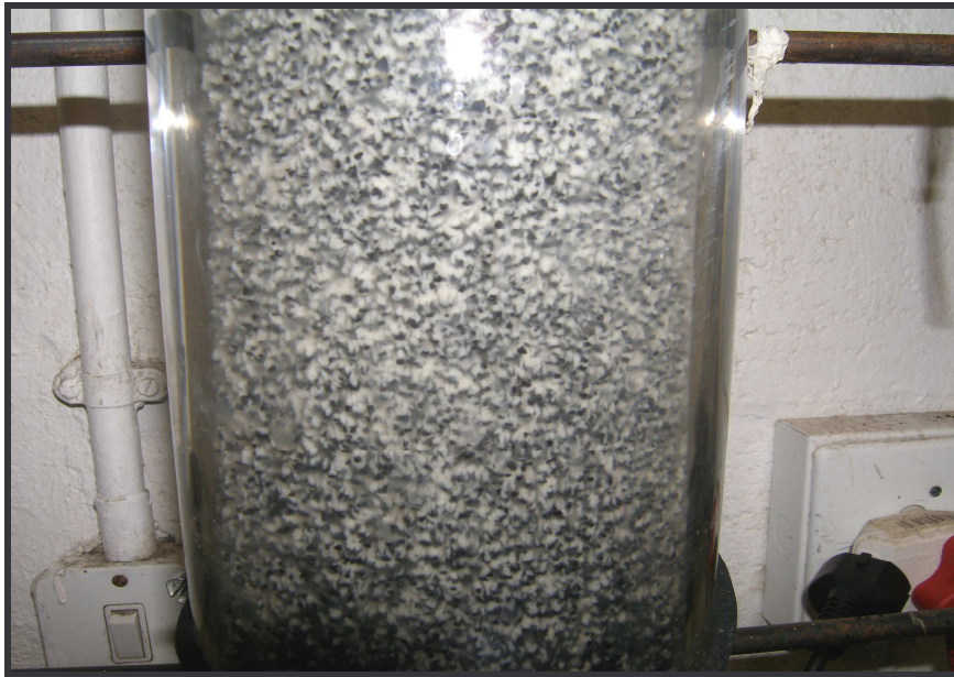
Figure 13 GAC coated with mixed undefined bacteria biofilm at 0.5 h HRT during the anaerobic FBBR operation
