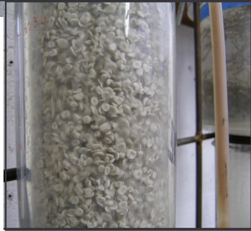
Figure 6 GAC coated by biofilm with carrier induced granules into the anaerobic FBBR inoculated with Ecl and Cf1 at HRT of 0.5h
