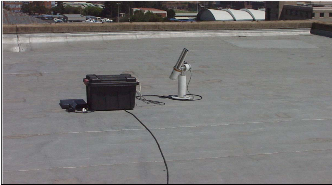
Figure 2.4: The CIMEL sun photometer situated at the University of the Witwatersrand
