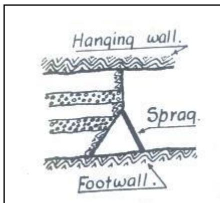
Figure 2.4 - Spragging of face of pillar, Crown Mines. 19
