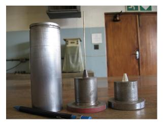
Figure 5.2 Mould for preparing specimens
