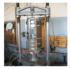
Figure 6.1 Apparatus for testing UCS
