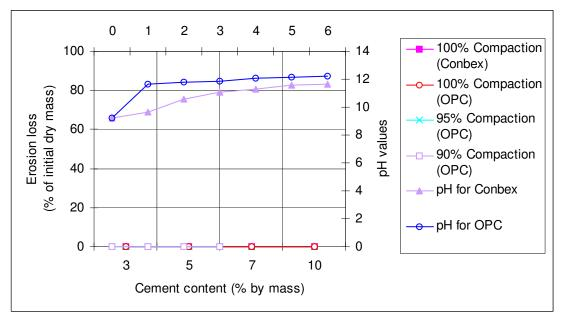
Figure 5.9 Analyses of the pinhole test for 7-days cured Kimberlite (C2) tailings
