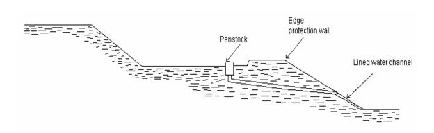
Figure 3.9 Erosion catchments berms (Chamber of Mines, 1996)
