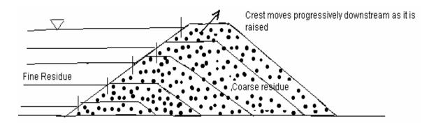
Figure 3.4 Downstream tailings dam construction (Klohn, 1980 and Blight, 1996).
