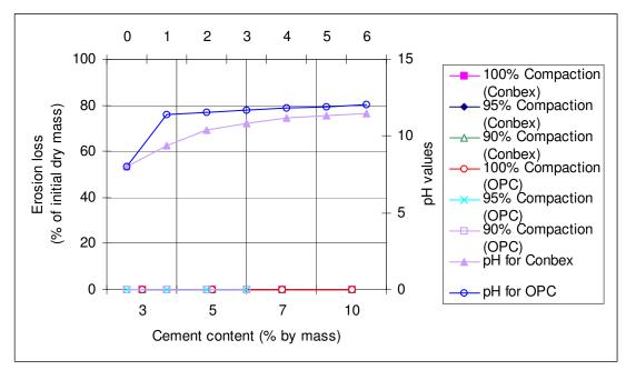
Figure 5.9 Analyses of the pinhole test for 7-days cured Kimberlite (C1) tailings
