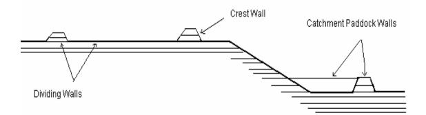
Figure 3.8 Crest walls and catchments paddock walls (Chamber of Mines, 1996)
