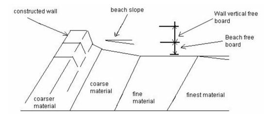
Figure 3.7 Principles of Spigot Deposition (Chamber of Mines, 1996)
