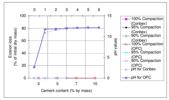
Figure 5.8 Analyses of the pinhole test for 7 days cured platinum tailings
