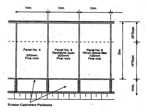
Figure 3.11 Port layout of large-scale erosion experiment (Blight and Amponsah-Dacosta, 2004).
