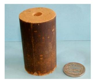
Figure 5.3 Pinhole specimens for gold tailing
