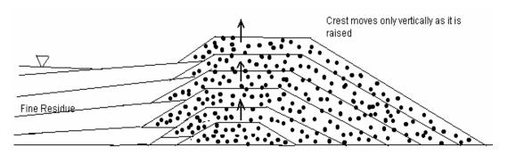
Figure 3.5 Centreline tailings dam construction (Klohn, 1980 and Blight 1996).
