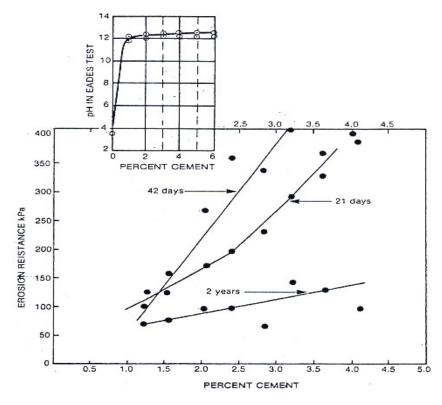
Figure 3.10 Results of tests on the stabilization of gold tailings with Portland cement (Blight and Caldwell, 1984).
