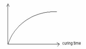
Figure 5.1 Illustration of strength development in cement stabilised materials
