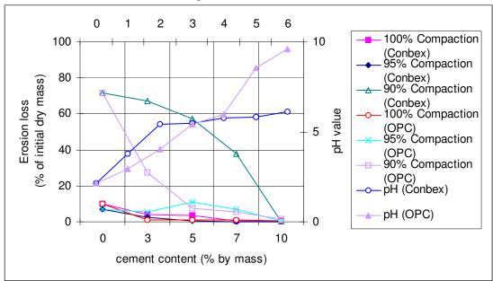
Figure 5.6 Analyses of the pinhole test for non-cured gold tailings
