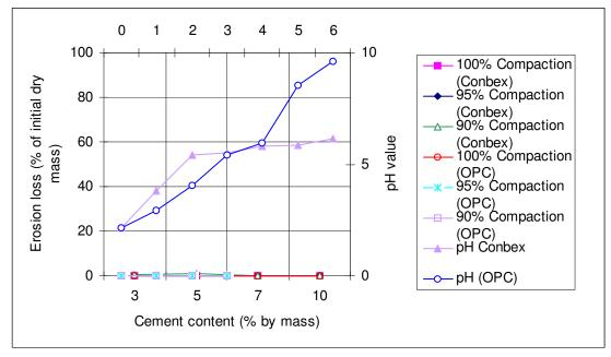
Figure 5.7 Analyses of the pinhole test for 7 days cured gold tailings
