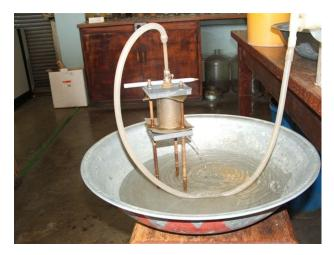
Figure 5.4 Set-up of the pinhole test
